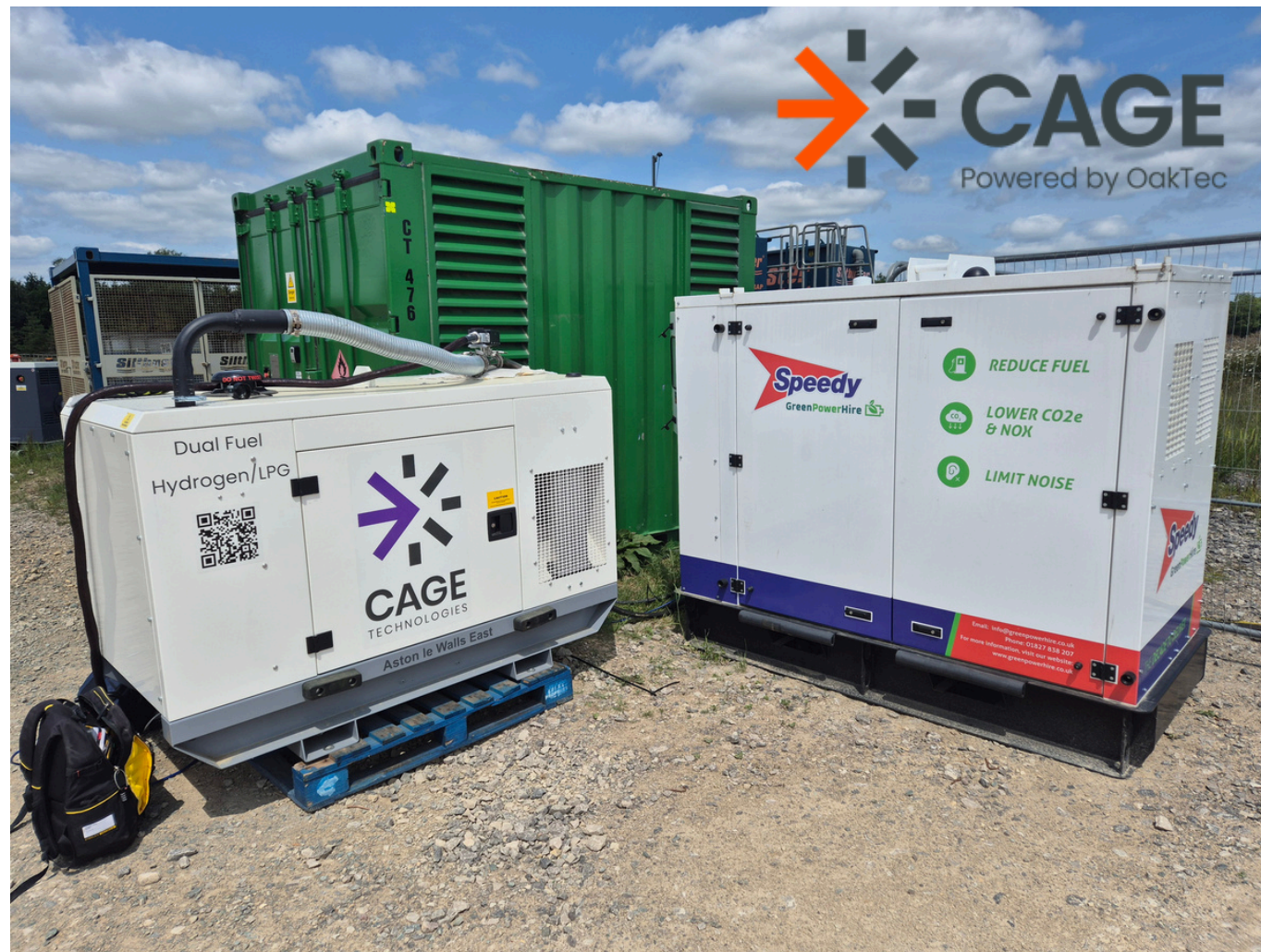
Multi-fuel generators – LPG/H2 Combustion 95% cleaner than diesel equivalent
